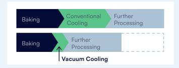
The necessary steam is created by reducing the pressure in the chamber: The lower the pressure, the lower the cooking point of water! The vacuum forces the water in the bread to continue to cook: On the one hand this allows the baking process to continue, on the other hand the energy needed for the cooking is taken from the bread. As a result, the bread is baked cold.
